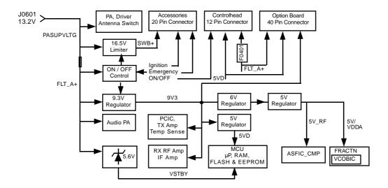
Figure 2-1 DC Power Distribution Block Diagram
