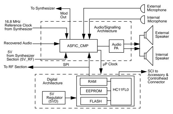
Figure 1-1 Controller Block Diagram
